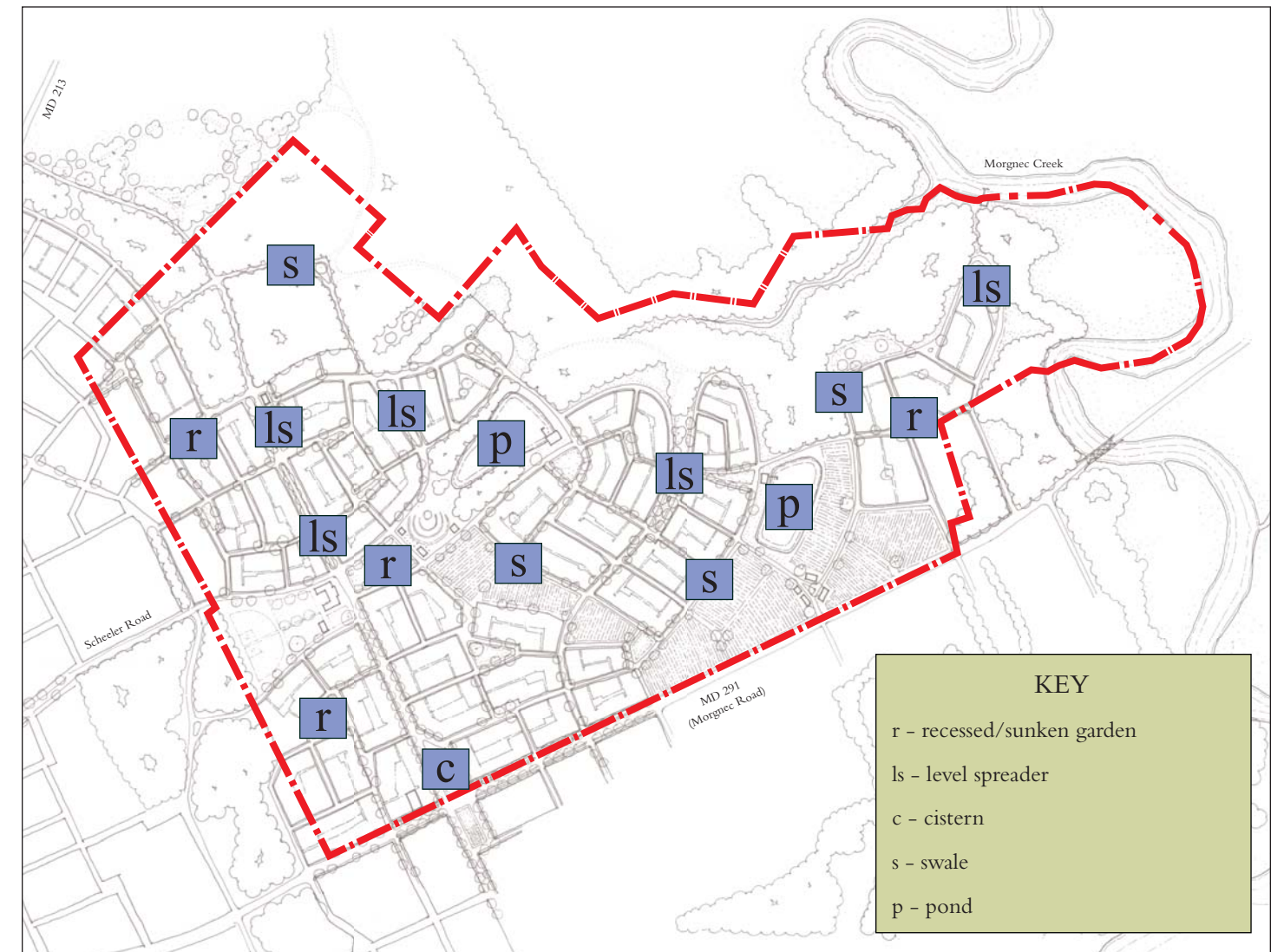
Rainwater management concept plan for Chestertown Greenbelt Master Plan featuring several plan and neighborhood scale options.
